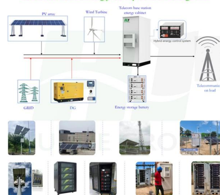
Base station energy composition diagram
